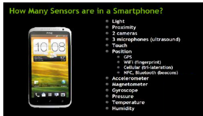
Figure 20 Sensors in a Typical Smartphone
